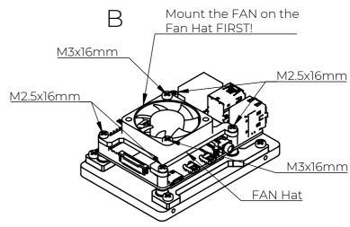
After mounting the fan, place the Pi and align it over the mounting holes. Then, place the fan hat and align it as well. Use the M2.5x16mm screws to secure it.
