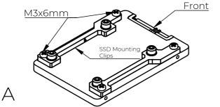
Place the drive on a flat surface and mount the SSD clips as shown above. Use M3x6mm screws to secure the SSD mounting clips. Please pay attention to the orientation.
