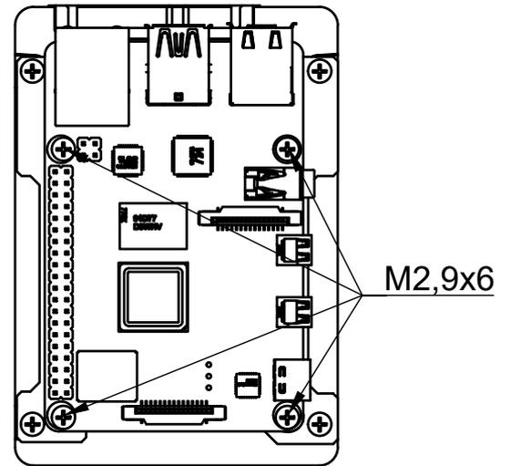
Place the Raspberry Pi over the mounting holes.
